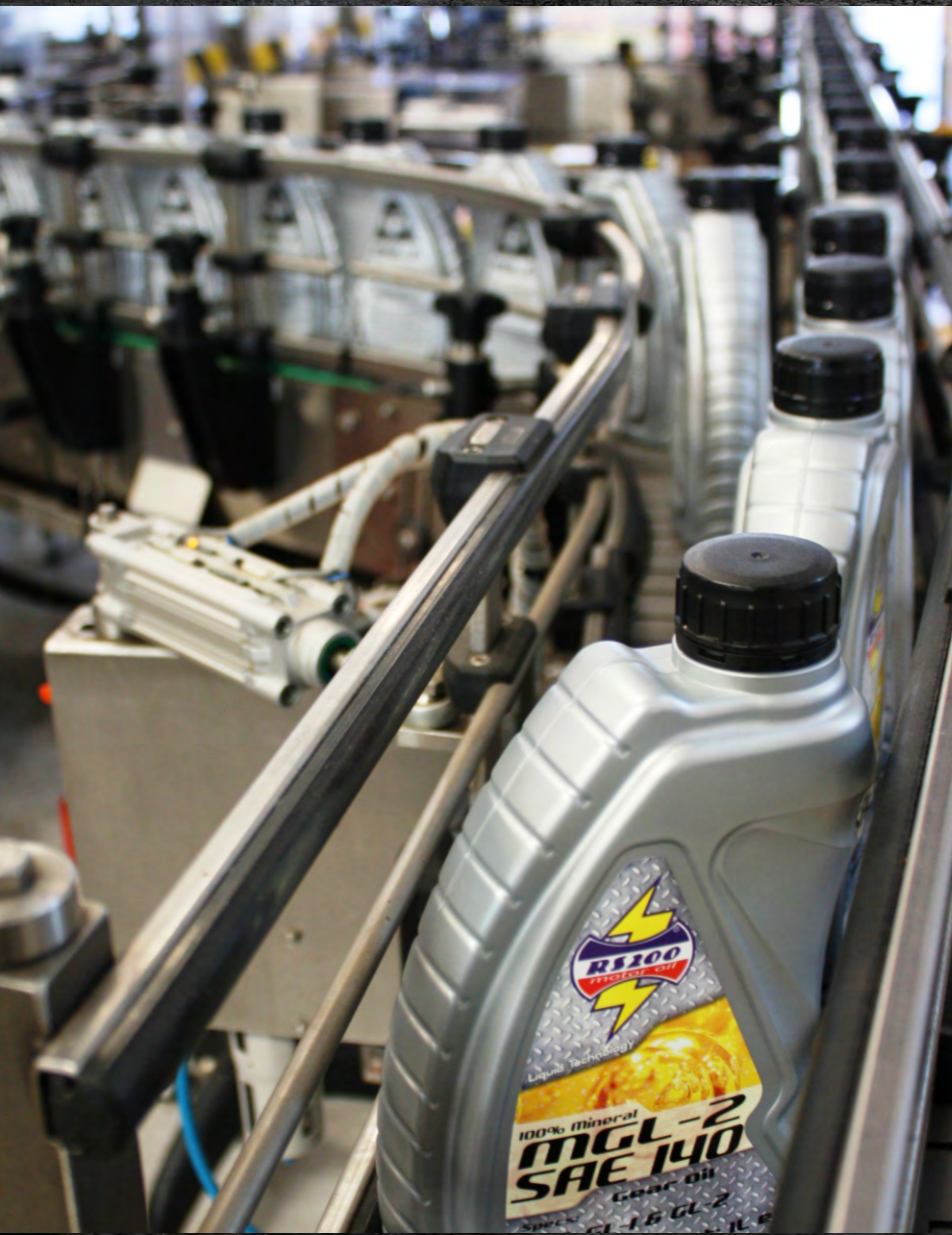
Photo of the production line (3.000bottles of 1L / hour)
